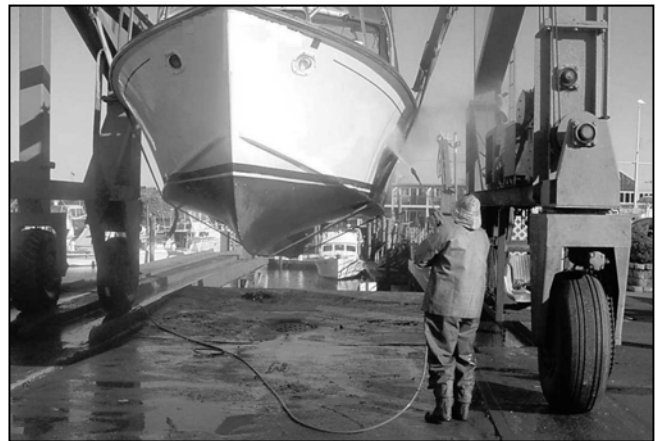
Figure 63. Pressure washing at a marina with a water collection and treatment system.
