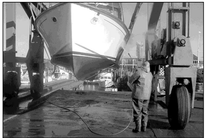
Figure 67. Pressure washing at a marina with a water collection and treatment system.
