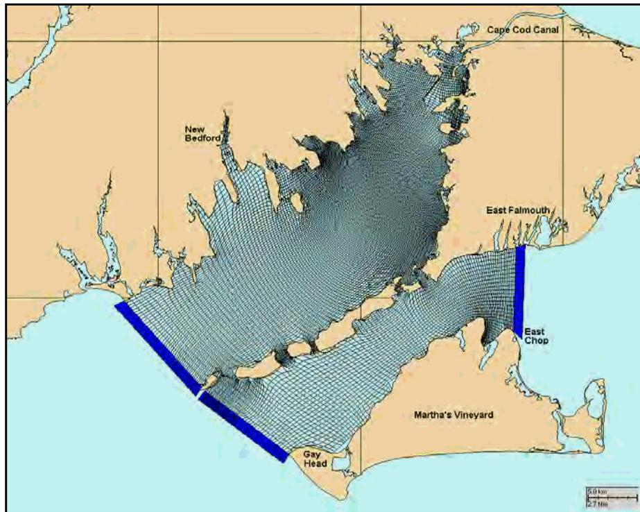
Figure B-4. Buzzards Bay oil spill model grid
