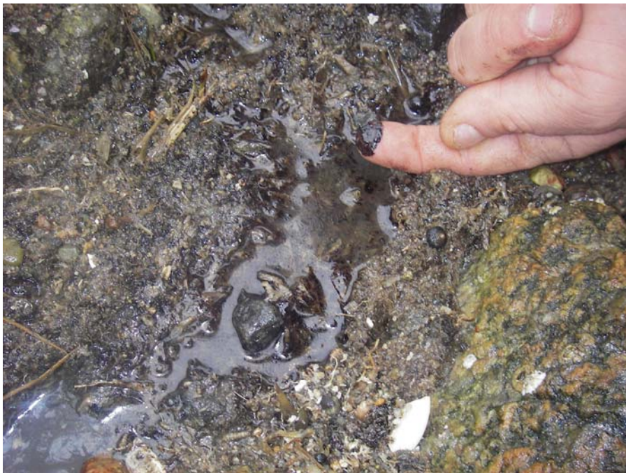
4. Liquid oil particles (floating on water surface) and sheen observed under a rock near the southern tip of Hoppy’s Landing.
