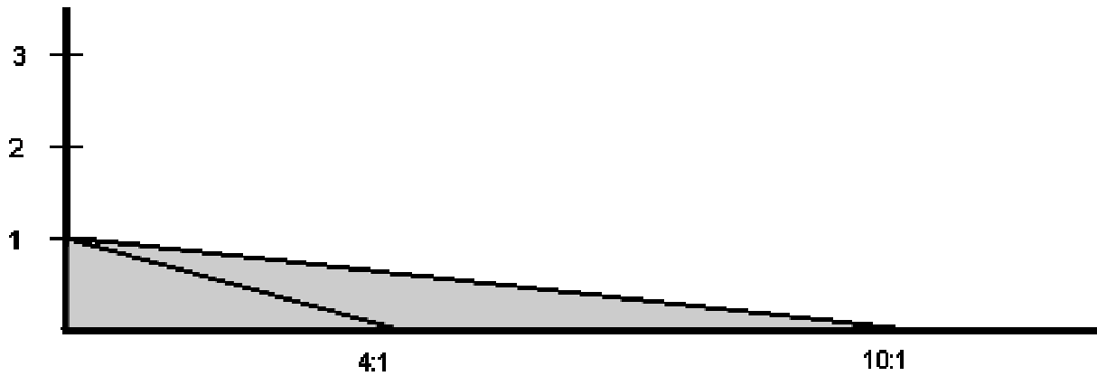
Figure 1: Note that a 4:1 slope is greater than (steeper than) a 10:1 slope.
