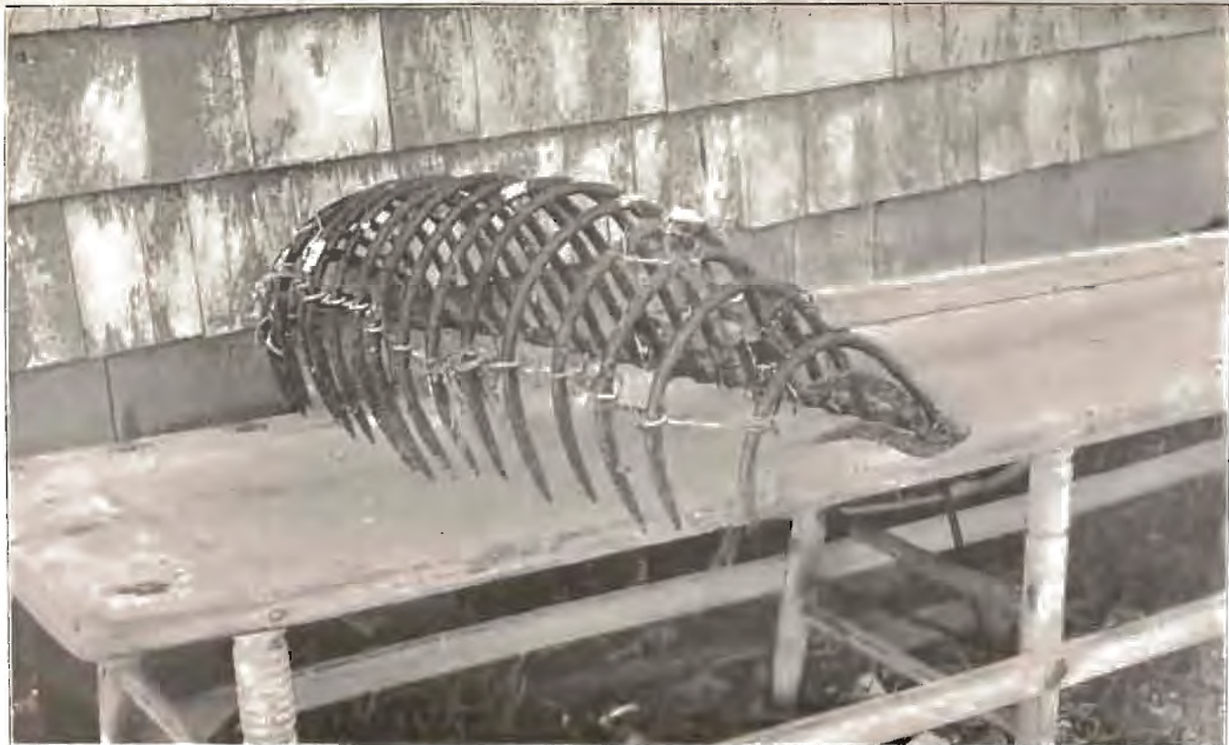
The Claw Quahaug Rake. — This rake varies greatly in size and length. Its use is chiefly confined to Nantucket. The general style has a handle 6 feet long, while the iron part, in the form of a claw or tub, with prongs 1 inch apart, is 10 inches wide. A heavier rake, as here shown, is sometimes used in the deeper water.
