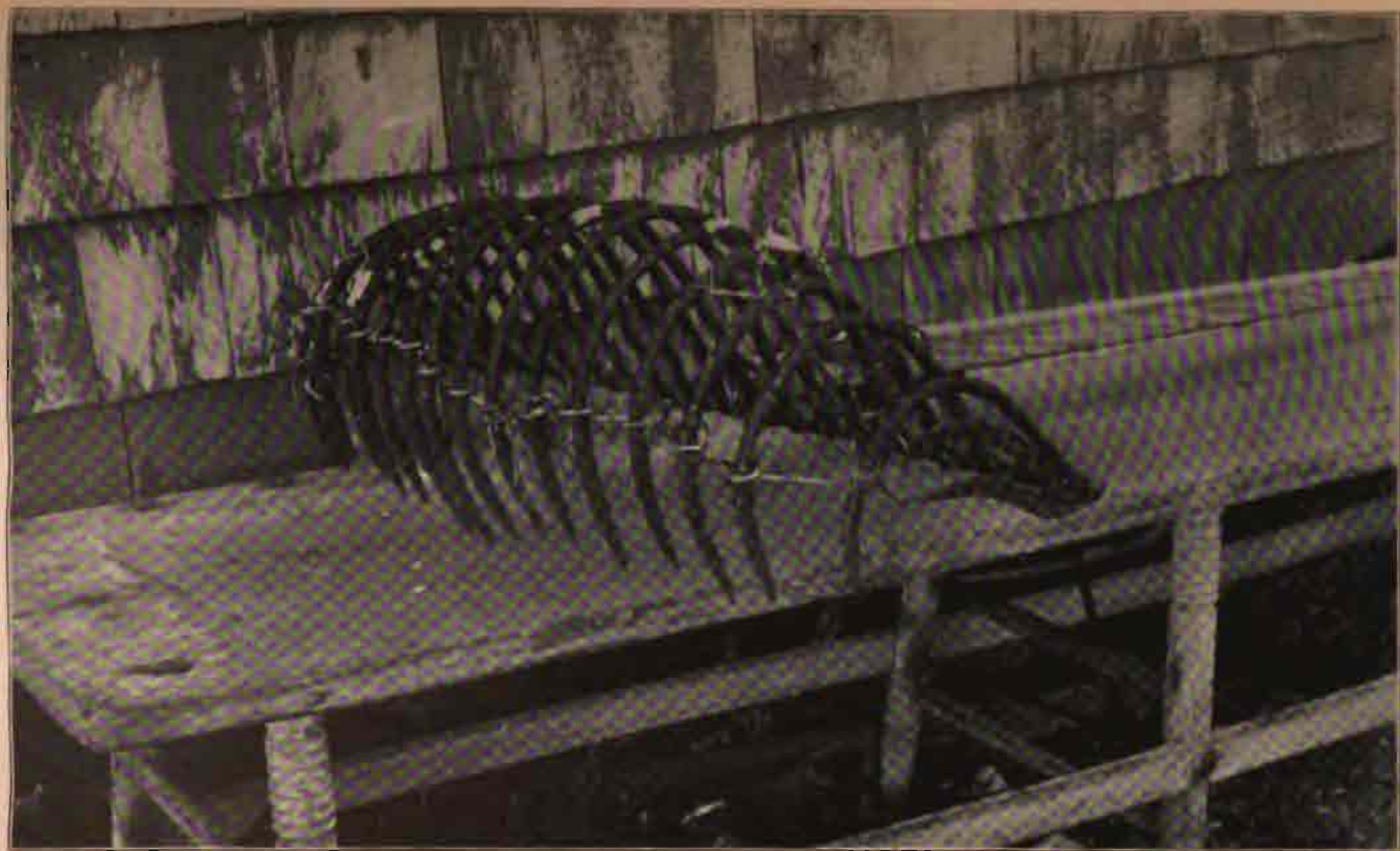
The Claw Quahaug Rake. — This rake varies greatly in size and length. Its use is chiefly confined to Nantucket. The general style has a handle 6 feet long, while the iron part, in the form of a claw or talon, with prongs 1 inch apart, is 16 inches wide. A heavier rake, as here shown, is sometimes used in the deeper water.
