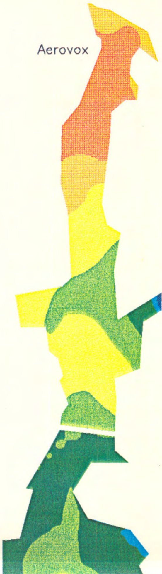
FIGURE 14. CONCENTRATION CONTOURS, AROCLOR 1248 IN SURFACE SEDIMENTS OF THE UPPER ACUSHNET ESTUARY
